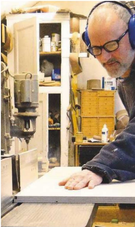
▲ Pic.6 Edward asked Richard if he would groove the table sides, the base and the top. "Nine mil any good?" he asked. His spindle moulder was set up to cut 9mm and it took seconds to adjust it and test it. Richard is deadly accurate. It's a powerful, and in his hands, precise machine. When he'd finished the top, he lowered the blade and took an extra sliver off so that the tongue would slide easily in the grooved sides. A second cut would take the whisper of wood remaining on this rebate
